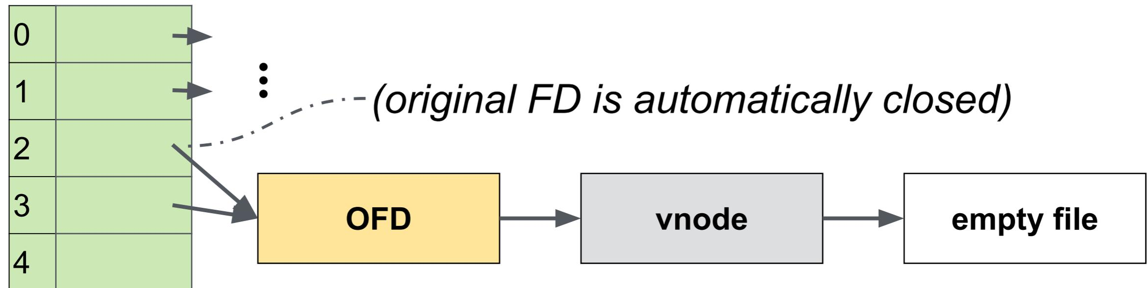
i.e., reading/writing FD 2 (*stderr*) is equivalent to doing so with FD 3
